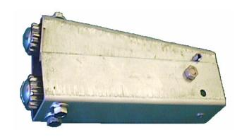
**TO USE THE CRIMPER** - Stand the frame on the end of the bench with the lug of the top bar over the edge. Lightly squeeze the wire between the rollers, and run the crimper down the wire. We suggest you do the top and bottom wires first, and then the other two.
